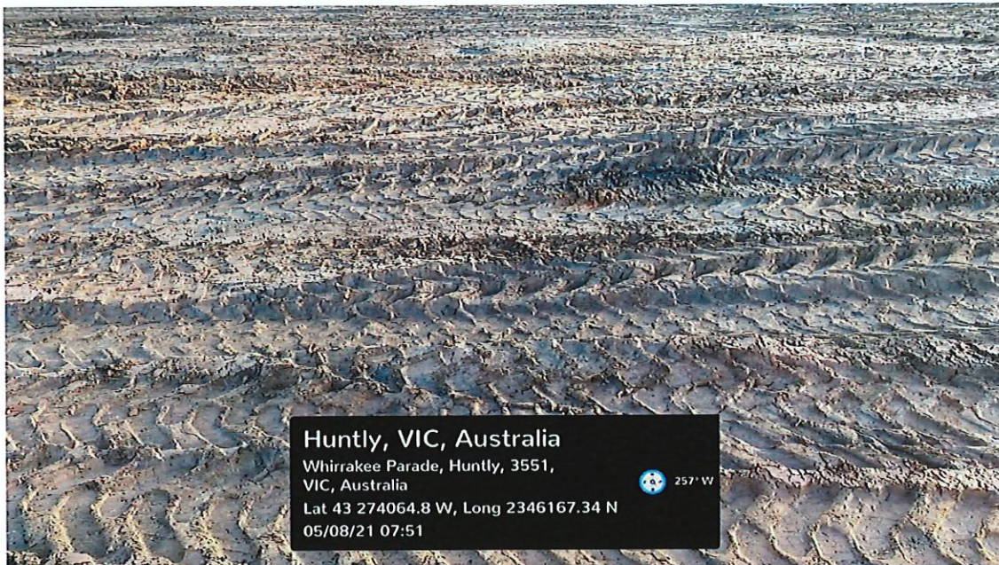
P2: Closer view of surface material and deformation under load to due moisture content
